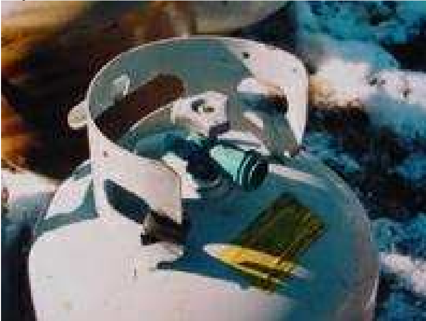
Figure 7 - Propane Tank Used for Methamphetamine Production (greening of valve caused by anhydrous ammonia)
