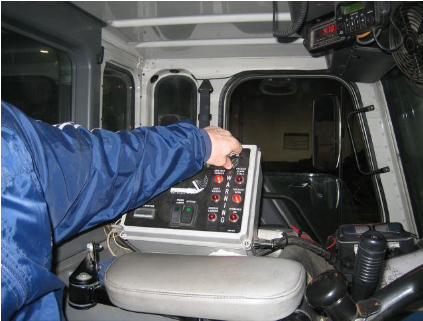
Fig 10: Accessing dump controls
