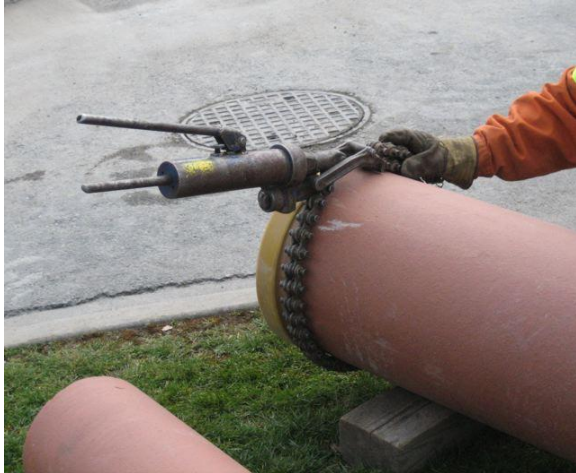
Fig 3: Pipe cutter for VIT pipe
