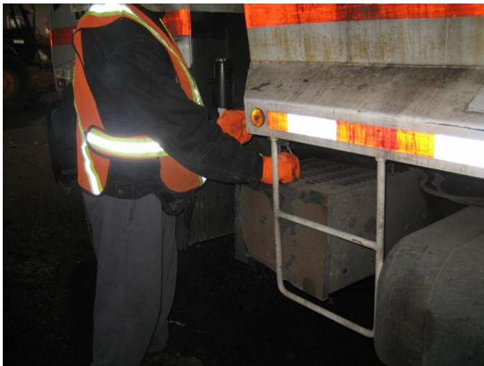
Fig 7: Operating dump controls
