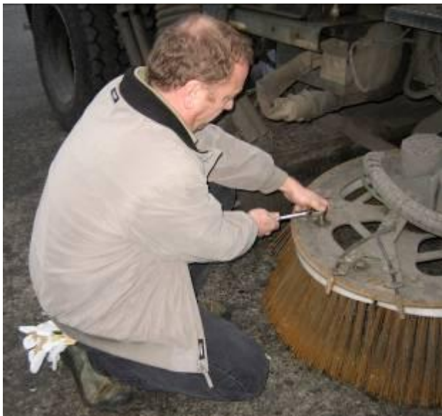
Fig. 5: Operator replacing gutter broom.
