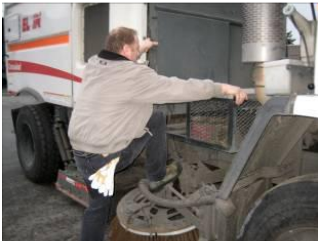
Fig. 3: Operator climbing onto the sweeper during pre-trip inspection.
