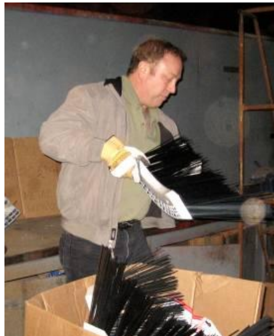
Fig. 6: Operator lifting new broom segments to replace gutter broom.
