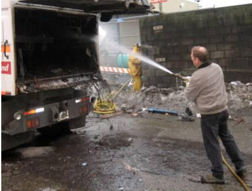
Fig. 9: Rinsing out back of sweeper at wash rack.
