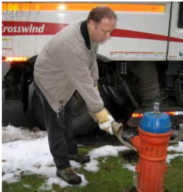
Fig. 7: Hooking up to a hydrant to fill the sweeper.
