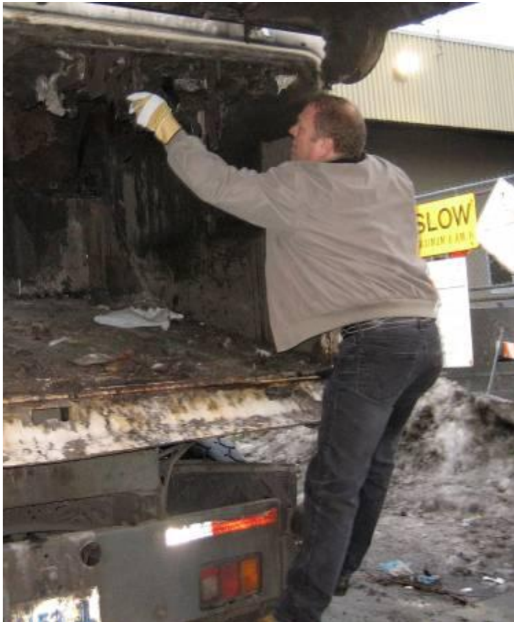
Fig. 10: Opening screens in rear of sweeper to rinse them.
