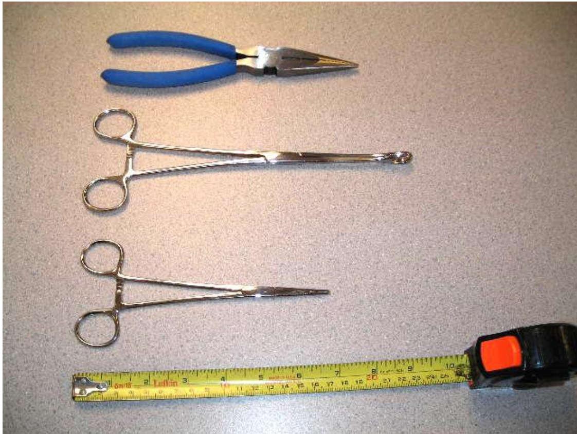
Figure 4: Long-nosed pliers or short or long forceps can be used to pick up needles. The employee has to stop or bend over when using these tools to pick up needles.
