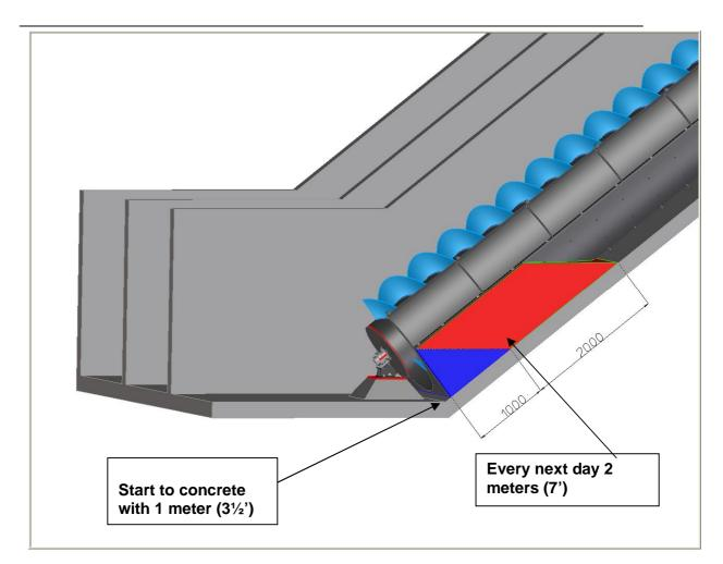
When the trough is finished, the spacers between trough and screw must be removed, the red brackets on the lower bearing must be removed and anchor bolts of the lower bearings must be tightened.
