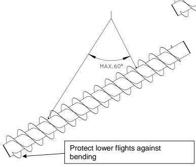
In case of using only one crane, great care will have to be taken, not to damage the flights of the screw. When the screw is tilted on the upper side, the screw can be leaning on the lower flights, which might be damaged in doing so.
