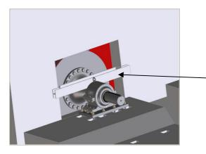
Example of a temporary support for the upper bearing (Not necessary for wall mounted bearings).
