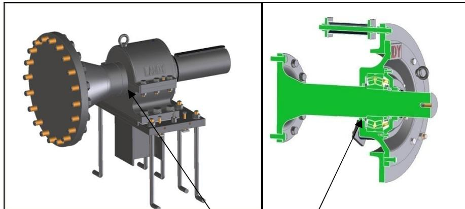
Clearance between shaft and housing at least 0.5mm (0.002") all around the shaft
