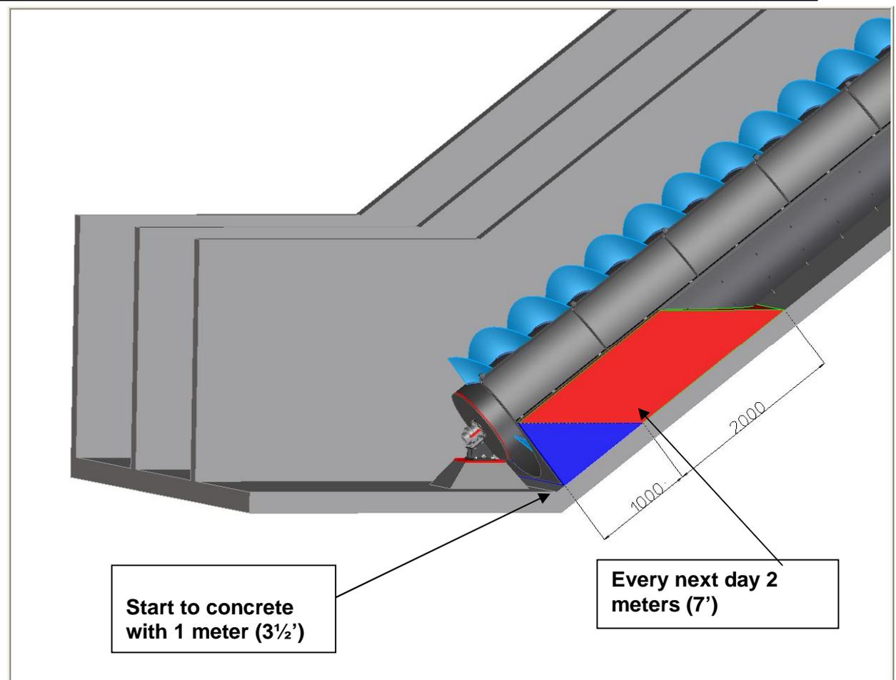
When the trough is finished, the spacers between trough and screw must be removed, the red brackets on the lower bearing must be removed and anchor bolts of the lower bearings must be tightened.
