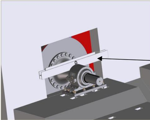
Example of a temporary support for the upper bearing (Not necessary for wall mounted bearings).
