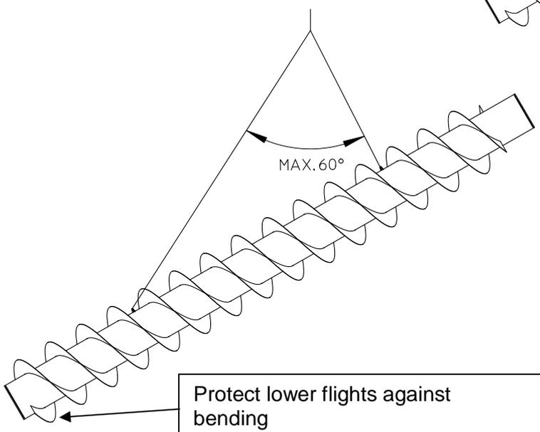
In case of using only one crane, great care will have to be taken, not to damage the flights of the screw. When the screw is tilted on the upper side, the screw can be leaning on the lower flights, which might be damaged in doing so.
