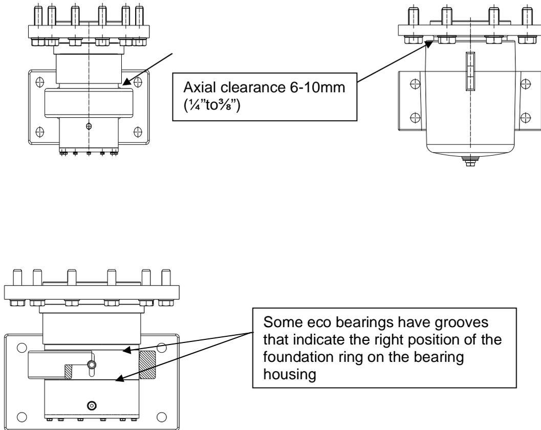
1. Check if the lower bearing has the right axial clearance. The forces of the weight of the screw pump and water will be taken by the upper bearing, The lower bearing must only support the screw radially, axial forces will destroy the lower bearing.
