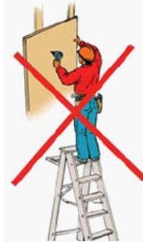
Workers must not work from the top two rungs of a ladder. Suitable hoisting equipment must be used for this purpose.
