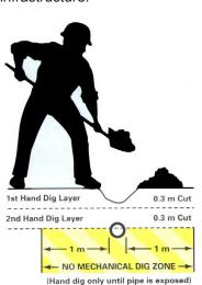
Once the utility or service is adequately exposed, mechanical digging is permitted to within 1 foot of the utility.
