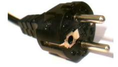
Always inspect cords before using. If there is any indication of damage, remove that piece of equipment or extension cord from use.
