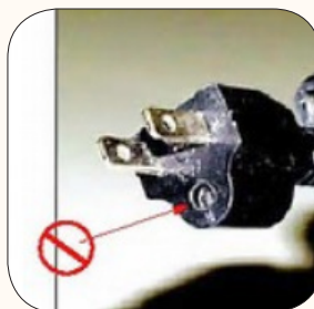
Ground removed from electrical cord
