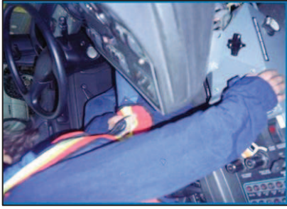
Figure 1: Releasing parking brake (push) while seated at the LEFT side: i) seat pushed to the back; ii) steering column tilted upwards; iii) steering wheel completely raised; iv) control panel pushed away from operator; v) shift buttocks to the right; and vi) arm on the side and elbow extended while pushing down on parking brake.
