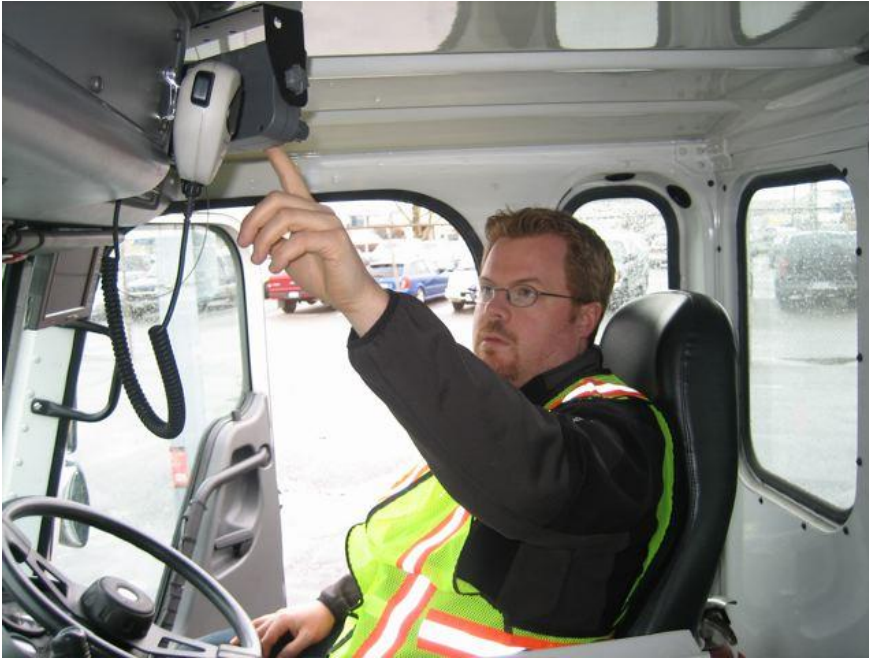
Fig 7: Accessing GPS unit
