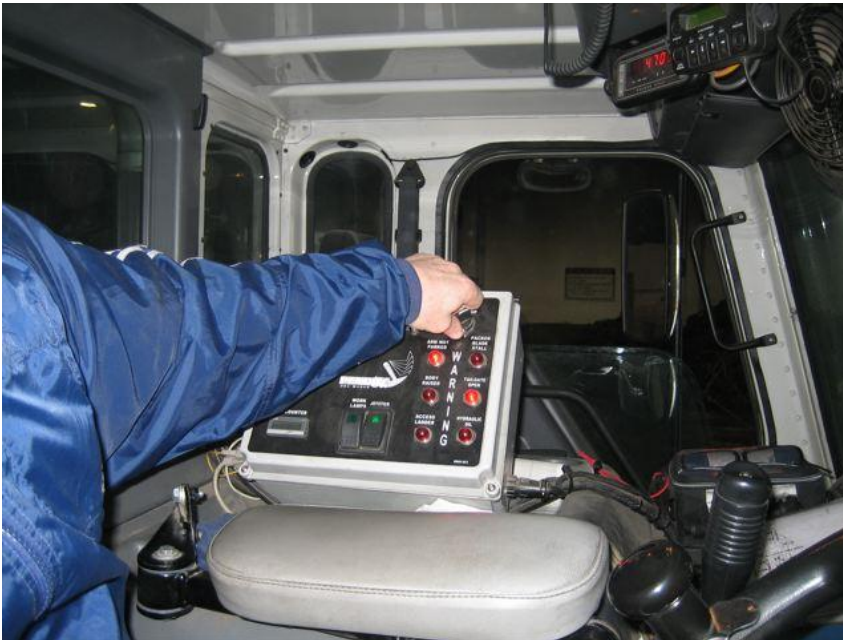
Fig 10: Accessing dump controls
