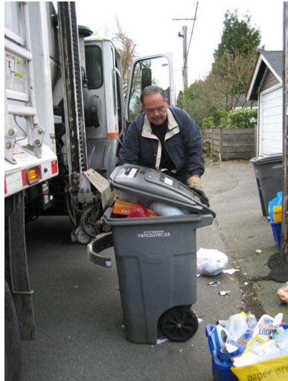
Fig 9: Manually positioning a tote
