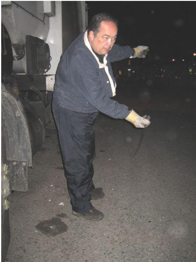
Fig. 2: Pre-Trip checking oil
