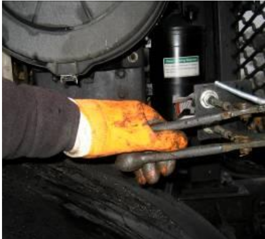
Fig. 5: Load controls on outside of truck.
