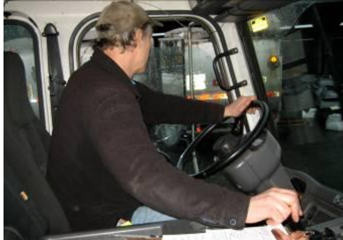
Fig. 6: Driver loading a container from inside the cab using mirrors and joystick.
