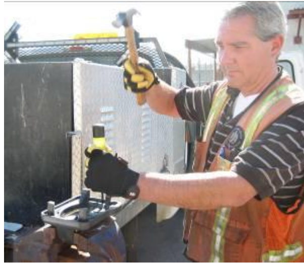
Fig. 4: Hammering stripped screws to replace a dome.
