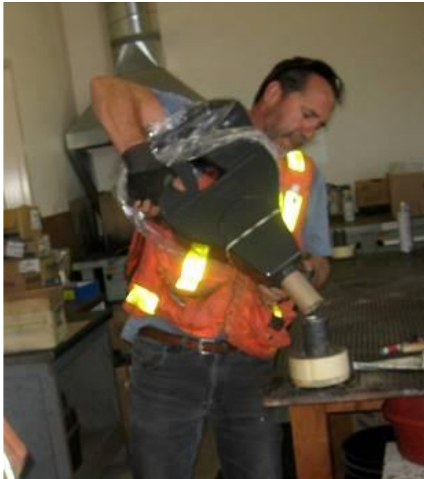
Fig. 16: Inserting new meter head into post on bench for assembly.
