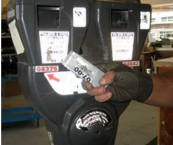
Fig. 6: Scraping illegible or out of date decals from a meter before reapplying.
