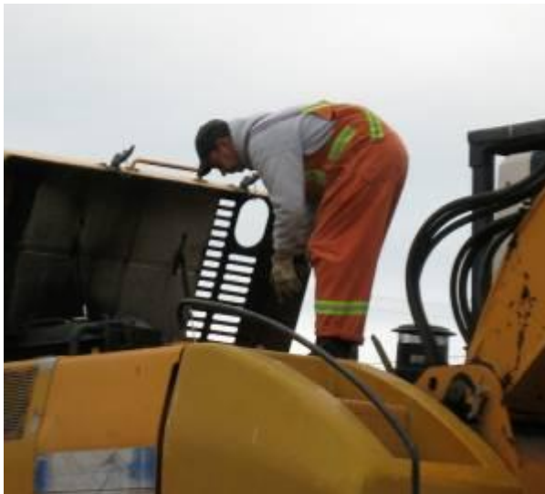
Fig 1: Ops II worker performing a pre-trip inspection on an excavator.
