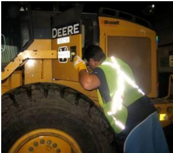
Fig. 1: Pre-trip inspection on loader.
