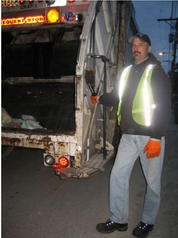
Fig 5: Operating tote lift and hopper controls.
