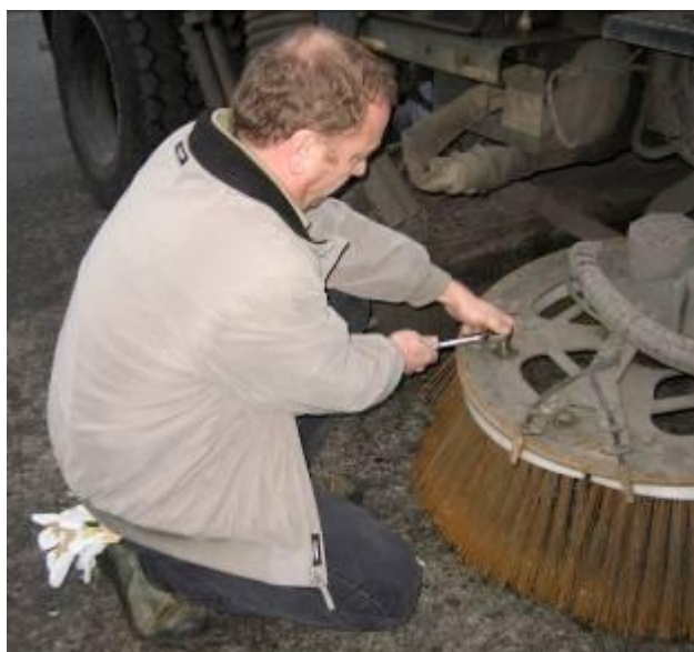
Fig. 5: Operator replacing gutter broom.
