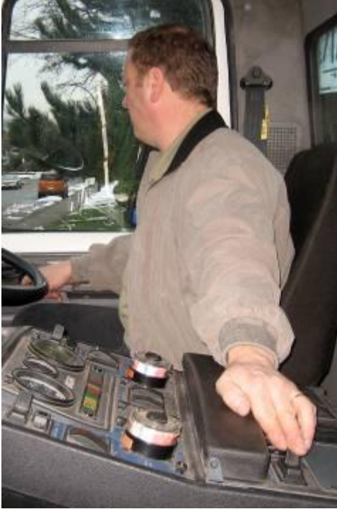
Fig. 1: Neck rotation to view gutter broom in mirror while operating controls.
