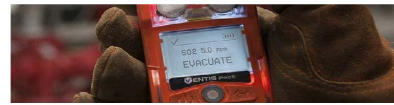
Gas detectors are lifesaving instruments that must be worn in your breathing zone to be effective. OSHA defines the breathing zone as "a hemisphere forward of the shoulders within a radius of approximately six to nine inches," so a collar, lapel, or outside breast pocket is usually a good option. This location also keeps the instrument visible so you can see alerts if your hearing is impaired while working in a high-noise environment.
